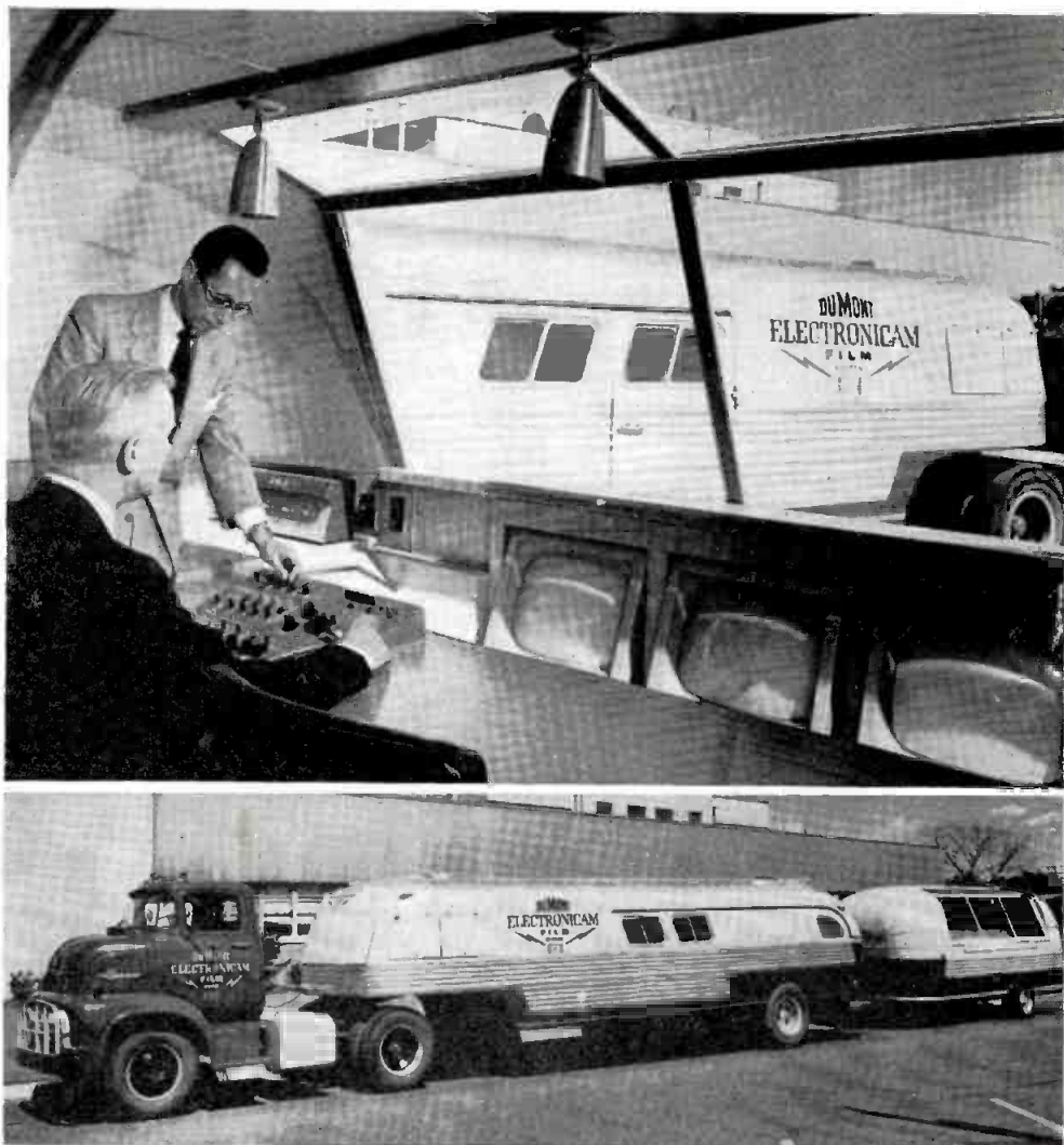
DUMONT'S new mobile Electronicam film system is contained in two functional trailers (bottom), readily moved from stage to stage and set to set. The smaller unit goes on stage as the control center while the larger one remains outside during film production. In the control-room trailer (top), the equipment is given a final check by Keeton Arnett (seated), vice president of Allen B. DuMont Labs, and John Auld, manager of operations, Electronicam Div., before unit leaves the Clifton, N. J., plant for use in Hollywood.
